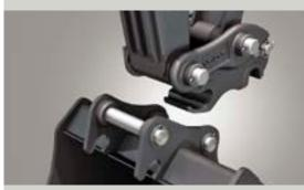
New pin-on Volvo attachment bracket.
