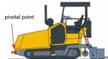
2. The screed transport cylinders push the screed downwards and raise the rear of the paver.
